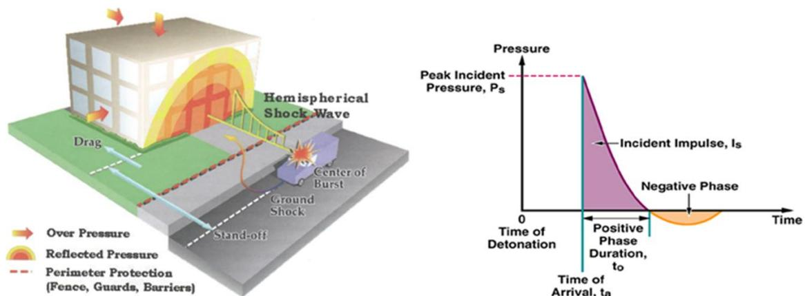
Figure 1. Schematic view of air-blast pressures acting on a building and pressure-time history of loading
