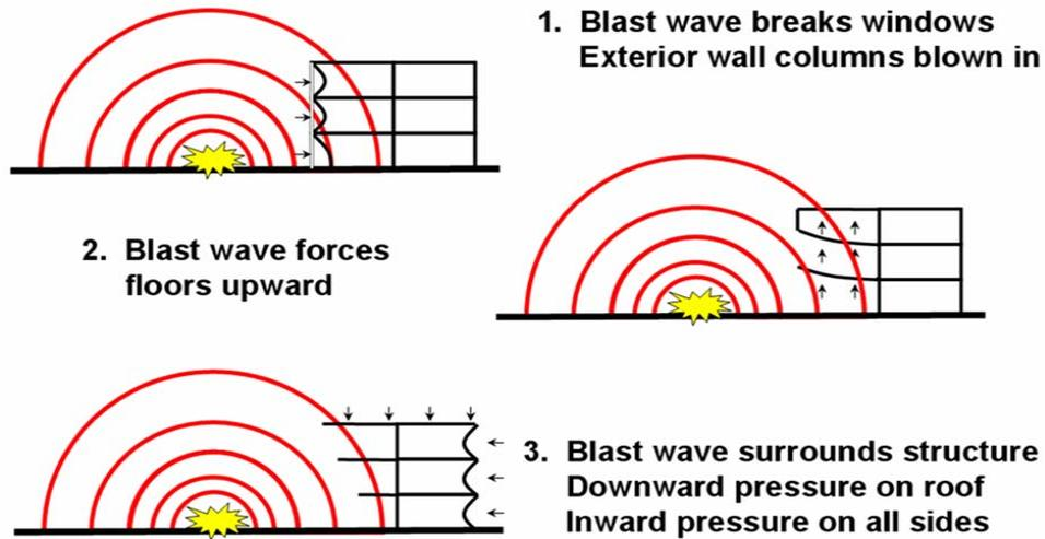
Figure 2. Damage pattern due to explosion
