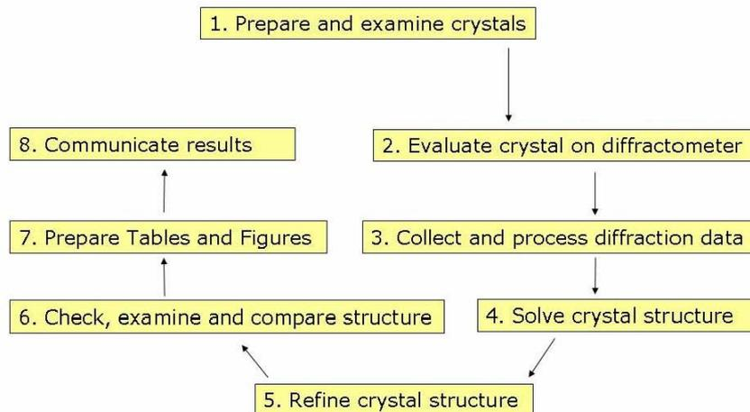
Figure 1. Outline of a typical single crystal structure determination.
