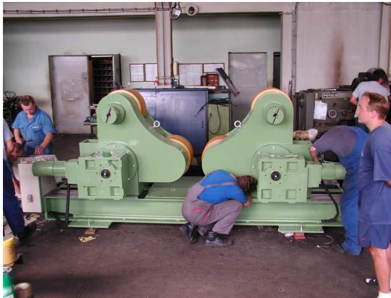
Figure 4. Power unit of 50 t “self-aligning” type Rotator, stable, Vulcolane rolls, tool spindle adjustment of blocks Courtesy: “Uniweld – strojevi”, Croatia
