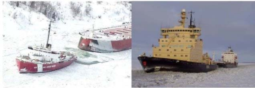
Figure 2. Early icebreakers had accommodation in the hull like the first USCGC Mackinaw (left). After 1970's the deck house replaced the superstructure like in the Finnish icebreaker Sisu (right).
