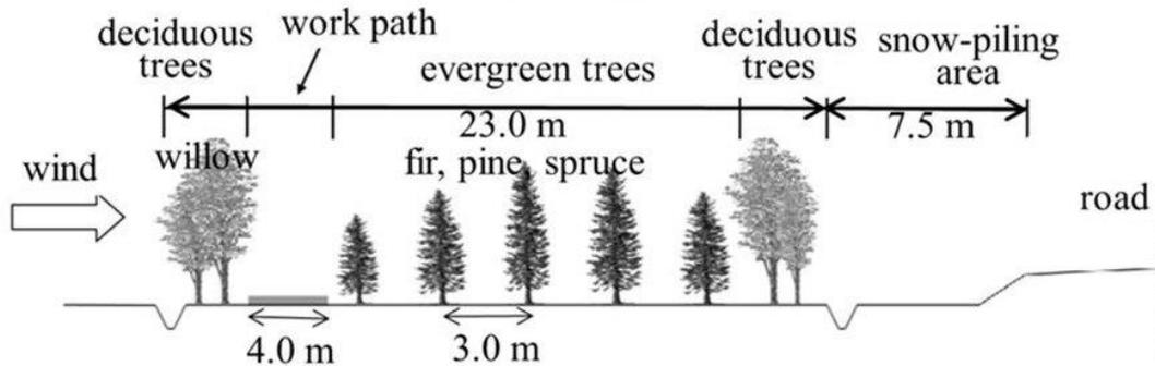
Figure 9. Basic structures of snow-break plantings (CERI, 2011)
