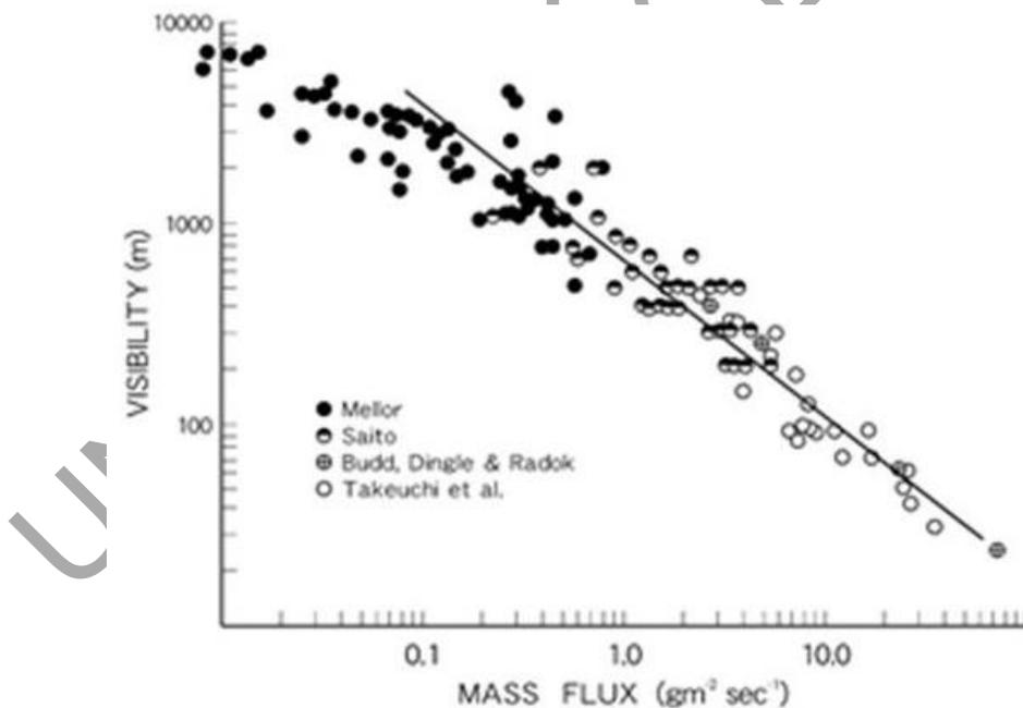
Figure 3. Relations between the mass flux of snow and visibility
