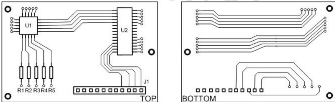
Figure 4. TOP and BOTTOM Sides (Layers) of a Sample PCB with Components and Traces.
