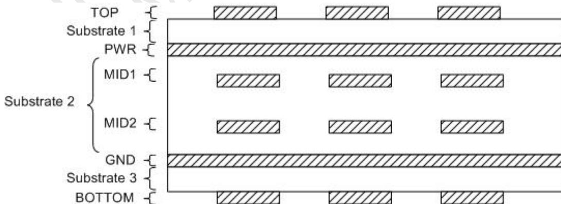
Figure 5. A 6-layer board stackup. Signals are routed on Top, Bottom, Mid1 and Mid2 layers.
