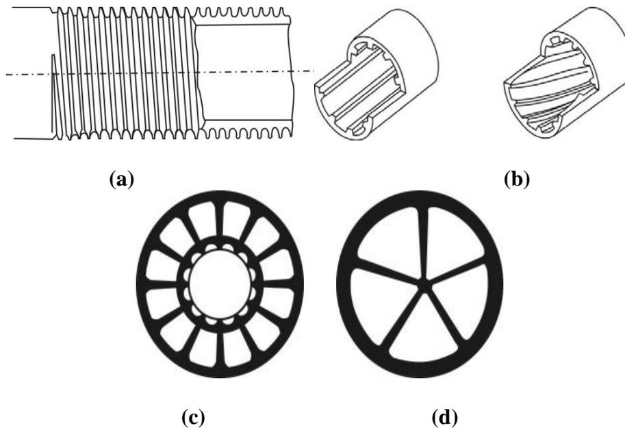
Figure 2. (a) Integral fins on outer tube surface (b) Internally finned tubes (axial and helical fins) (c) Cross sections of multiply internally finned tubes (d) tube with aluminum star insert [From Webb, R. L. and Kim, N. H., 2005, *Principles of Enhanced Heat Transfer*, Taylor & Francis, NY, USA, 2nd Edition.]
