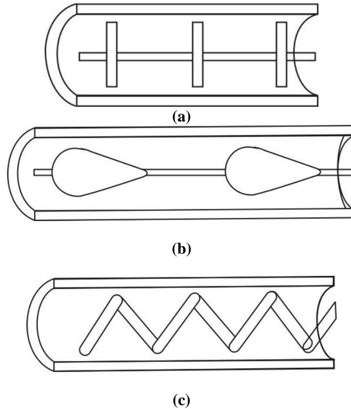
Figure 3. (a) Spaced disk devices (b) Spaced streamline-shaped insert devices (c) Displaced wire-coil insert [From Webb, R. L., 1987, *Enhancement of Single-Phase Heat Transfer*, Handbook of Single Phase Heat Transfer, S. Kakac, R. K. Shah and W. Aung, Eds., John Wiley and Sons, NY, USA.]
