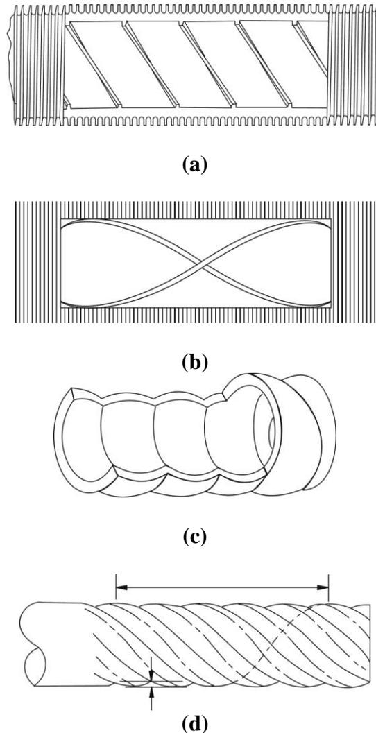
Figure 4. Methods used to make doubly enhanced tubes. (a) Helical rib roughness on inner surface and integral fins on outer surface, (b) Insert device (twisted tape) with integral fins on outer surface, (c) Corrugated inner and outer surfaces, (d) Corrugated strip rolled in tabular form and seam welded. [From Webb, R. L., 1987, *Enhancement of Single-Phase Heat Transfer*, Handbook of Single Phase Heat Transfer, S. Kakac, R. K. Shah and W. Aung, Eds., John Wiley and Sons, NY, USA.]
