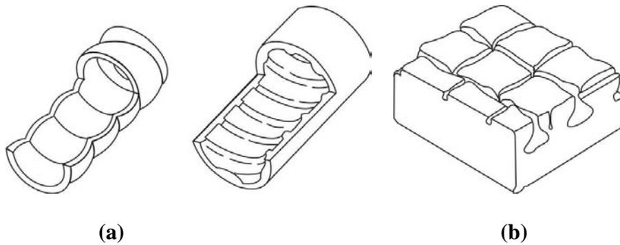
Figure 1. (a) Tube side roughness for single-phase or two phase flow (b) rough surface for nucleate boiling [From Webb, R. L. and Kim, N. H., 2005, *Principles of Enhanced Heat Transfer*, Taylor & Francis, NY, USA, 2nd Edition.]
