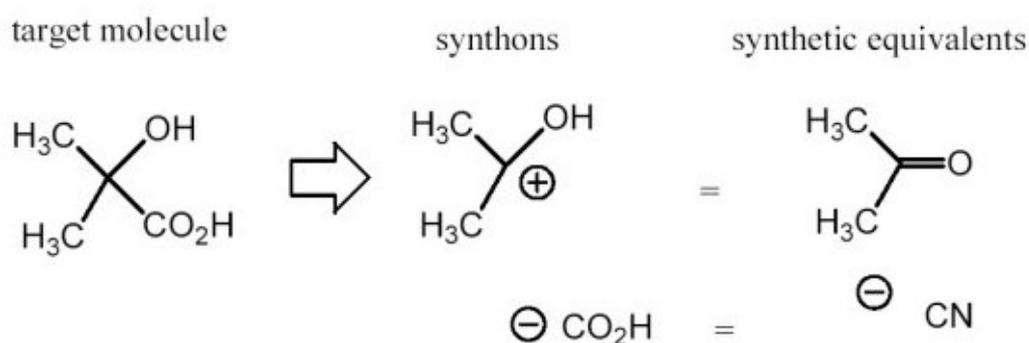
Figure 5: A simple disconnection: the cyanide ion is the synthetic equivalent of the  $^-\text{COOH}$  synthon.
