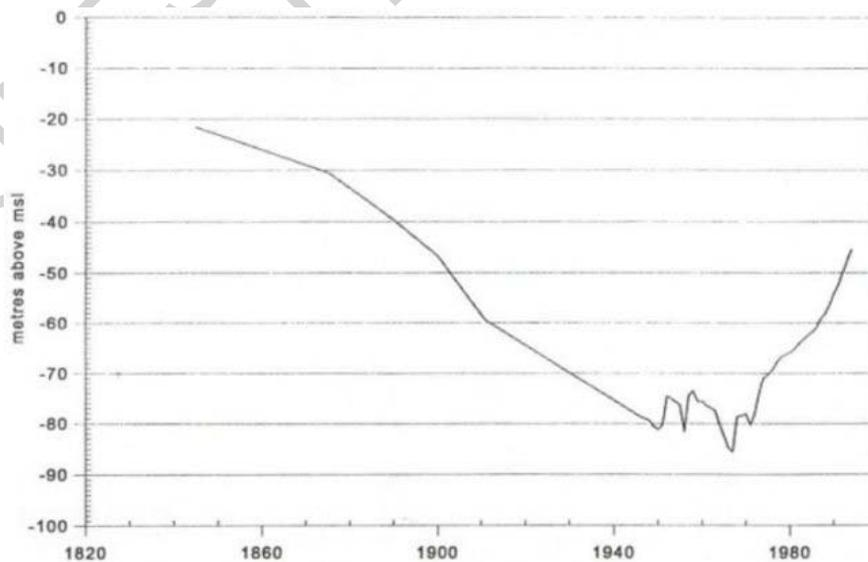
Figure 2. Falling and rising of the groundwater level evolution in the chalk aquifer underlying London
