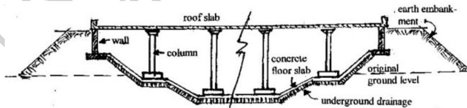
Figure 4(b). Vertical cross-section through a very large reinforced concrete reservoir of 50 to 500 megaliter capacity
