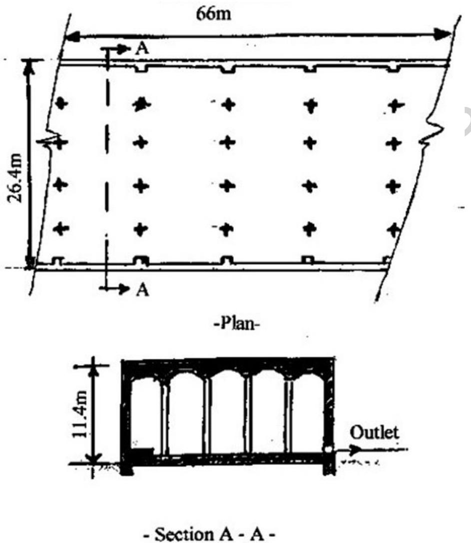
Figure 2(a). A Roman reservoir with vaulted roof supported by columns
