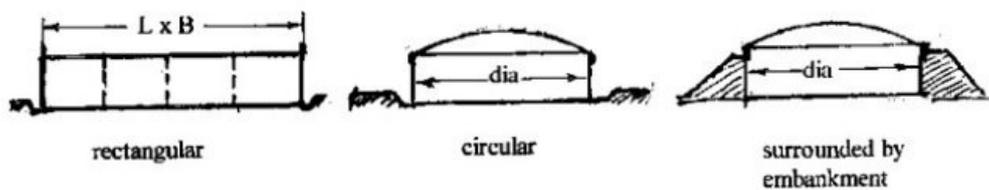
Figure 4(a). Typical 1 to 25 megaliter capacity reservoirs
