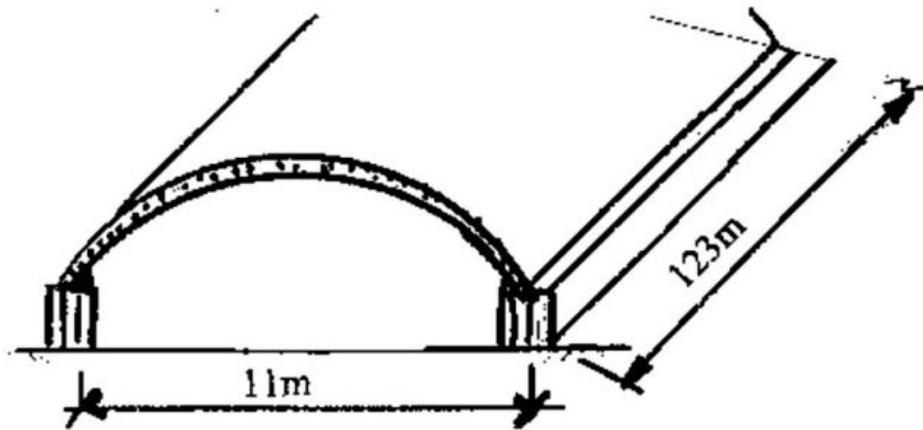
Figure 2(b). A Roman reservoir with barrel-vaulted chambers
