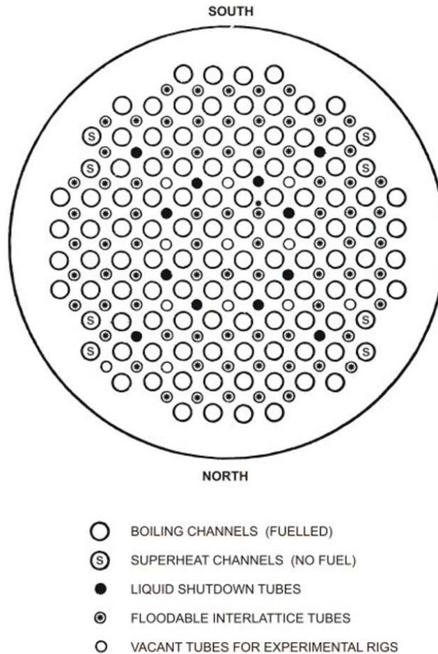
Figure 4. Reactor core plan view
