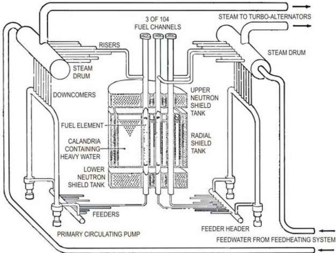
Figure 2. Reactor general arrangement
