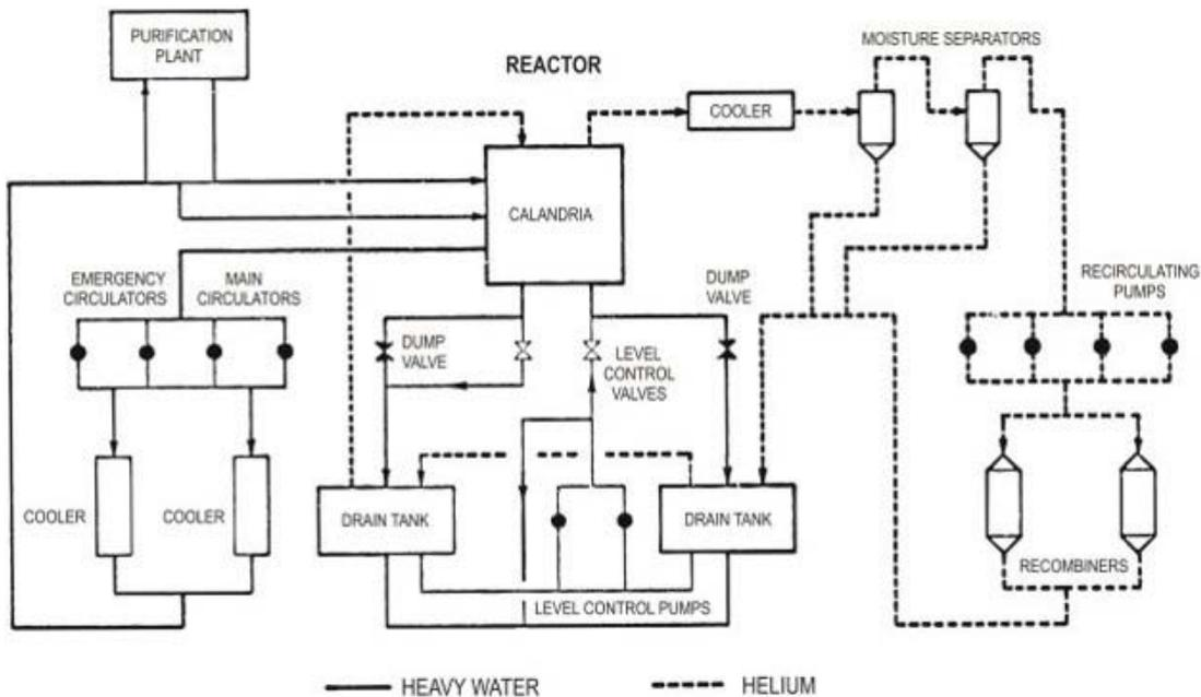
Figure 3. Heavy water moderator circuit
