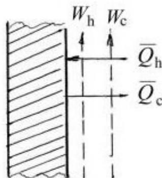
Figure 5. Schematic of the regenerative heat exchanger ( $\bar{Q}_h$  is the direction of the heat flux from a hot heat exchanger;  $\bar{Q}_c$  is the direction of the heat flux from a cold heat exchanger).
