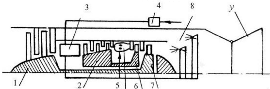
Figure 1. Schematic of the by-pass turbojet engine with reheat (TJER): 1 – fan; 2 – inner loop compressor; 3 – fuel-air heat exchanger; 4 – fuel pump; 5 – combustion chamber; 6 – compressor turbine; 7 – fan turbine; 8 – reheat chamber; 9 – propulsive nozzle.
