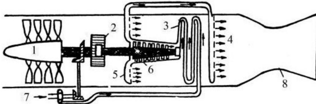
Figure 2. Schematic of the air-jet engine with the compressor drive from the superheated hydrogen turbine [8]: 1 – fan; 2 – reducer; 3 – heat exchanger; 4 – burning up chamber; 5 – turbine; 6 – main combustion; 7 – liquid hydrogen pump.
