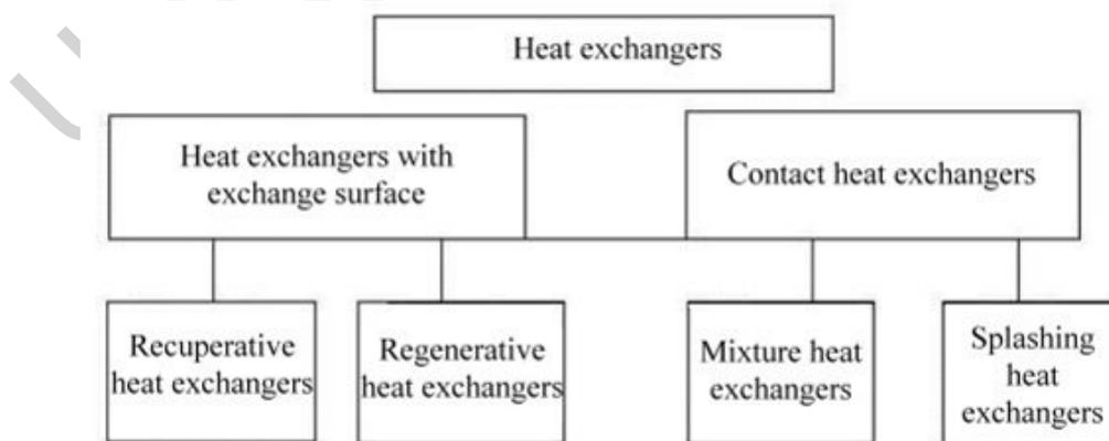
Figure 3. Classification of heat exchangers
