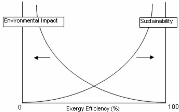
Figure 5. Qualitative illustration of the relation between the environmental impact and sustainability of a process, and its exergy efficiency.
