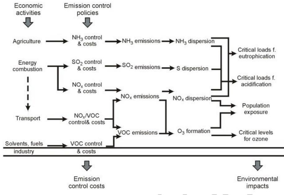
Figure 1. Schematic flowchart of the RAINS model framework
