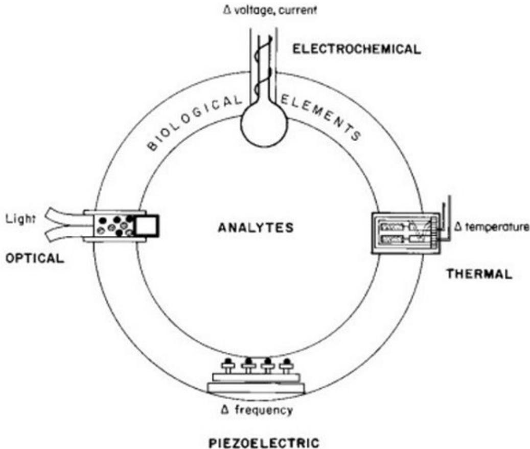
Figure 2: Transducers used in the construction of biosensors
