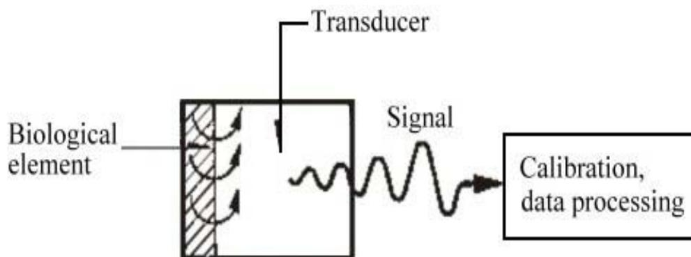
Figure 1: General concept of a biosensor
