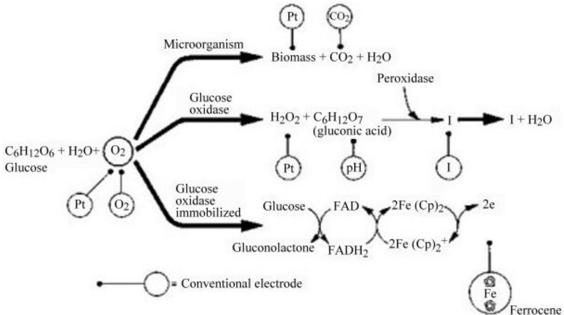
Figure 4: Alternative techniques for measuring glucose concentration using different biological elements and transducers
