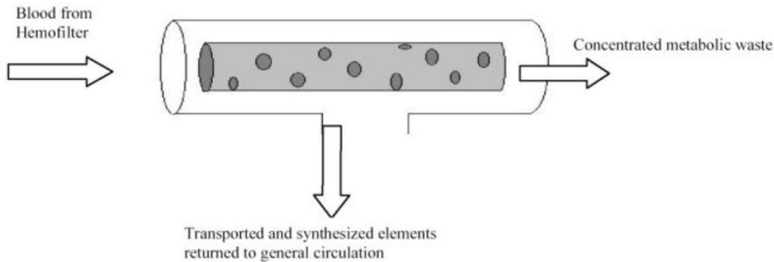
Figure 2. Single, hollow fiber bioartificial renal tubule. Renal tubule cells line porous polymer fibers, providing transport and metabolic function.
