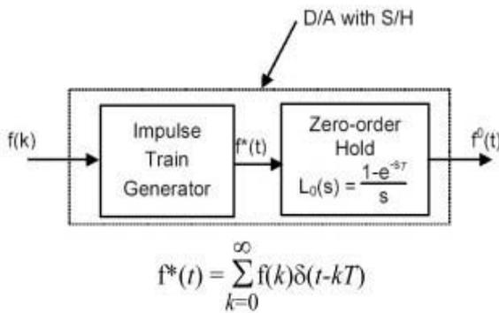
Figure 3: Digital-to-Analog (D/A) Conversion with Sample and Hold (S/H)
