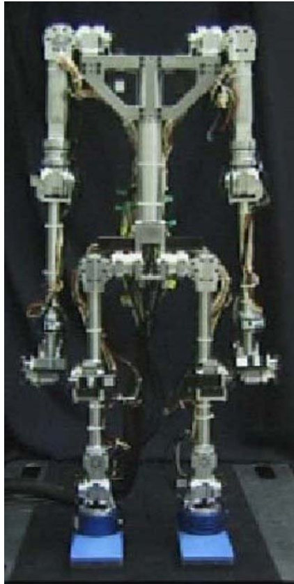
Figure 6 (c): Gorilla II- Multi-locomotive robot
