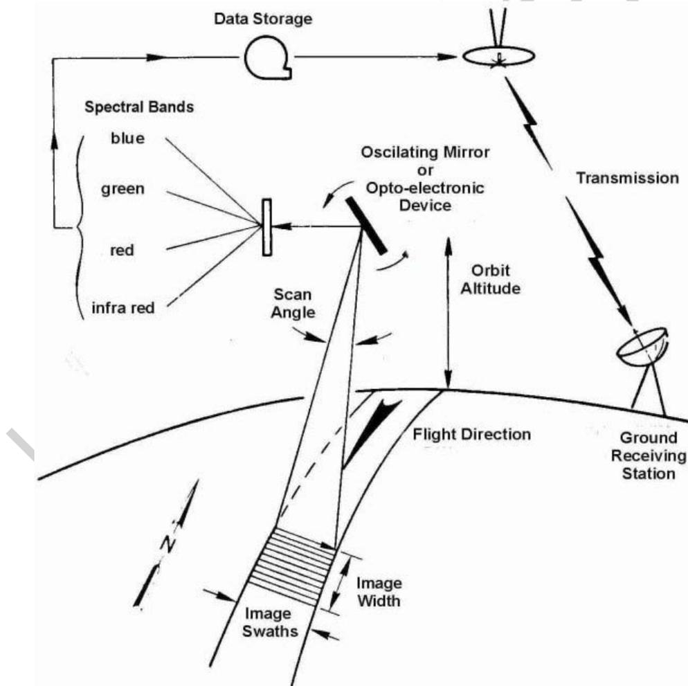
Figure 2. Principle of data recording, scanning process
