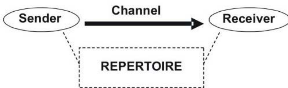
Figure 1. Schematic representation of the basic components of the simplest communication system.
