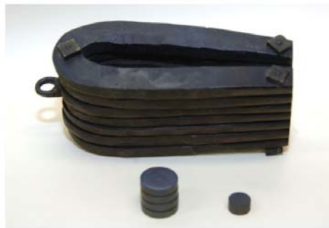
Figure 4: Illustration of three permanent magnets: an early steel magnet (top), hexagonal ferrite (bottom left) and a modern rare-earth permanent magnet (bottom right). Each magnet stores about the same amount of energy - a fraction of a joule.
