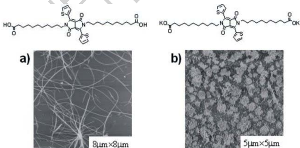
Figure 6. The AFM images of aggregation of bola-type amphiphile: a) with the terminal carboxyl acid groups; b) with the terminal potassium salt groups. Copyright 2007 WILEY-VCH Verlag GmbH & Co. KGaA, Weinheim.
