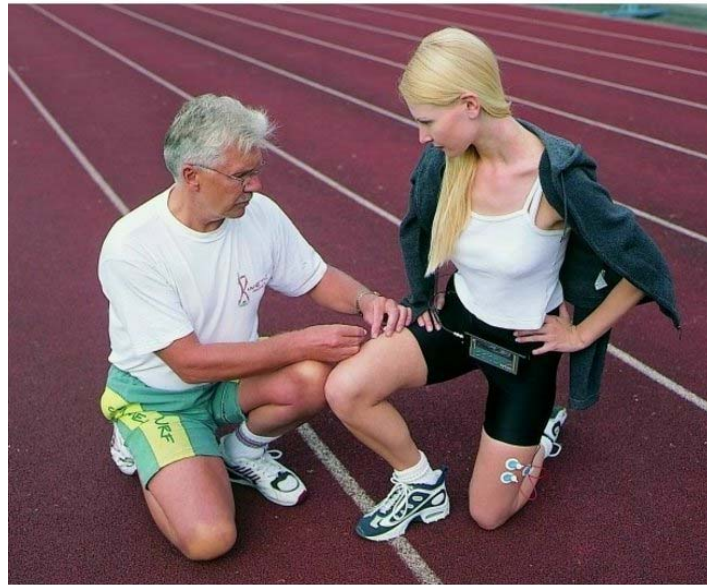
Figure 1. Measurement of the electrical activity of quadriceps femoris muscles of an athlete with a portable electromyograph. The coach is attaching the surface electrodes before the running test. Surface electrodes cause no pain and do not hamper the performance. The device stores the signals for later computer analysis.
