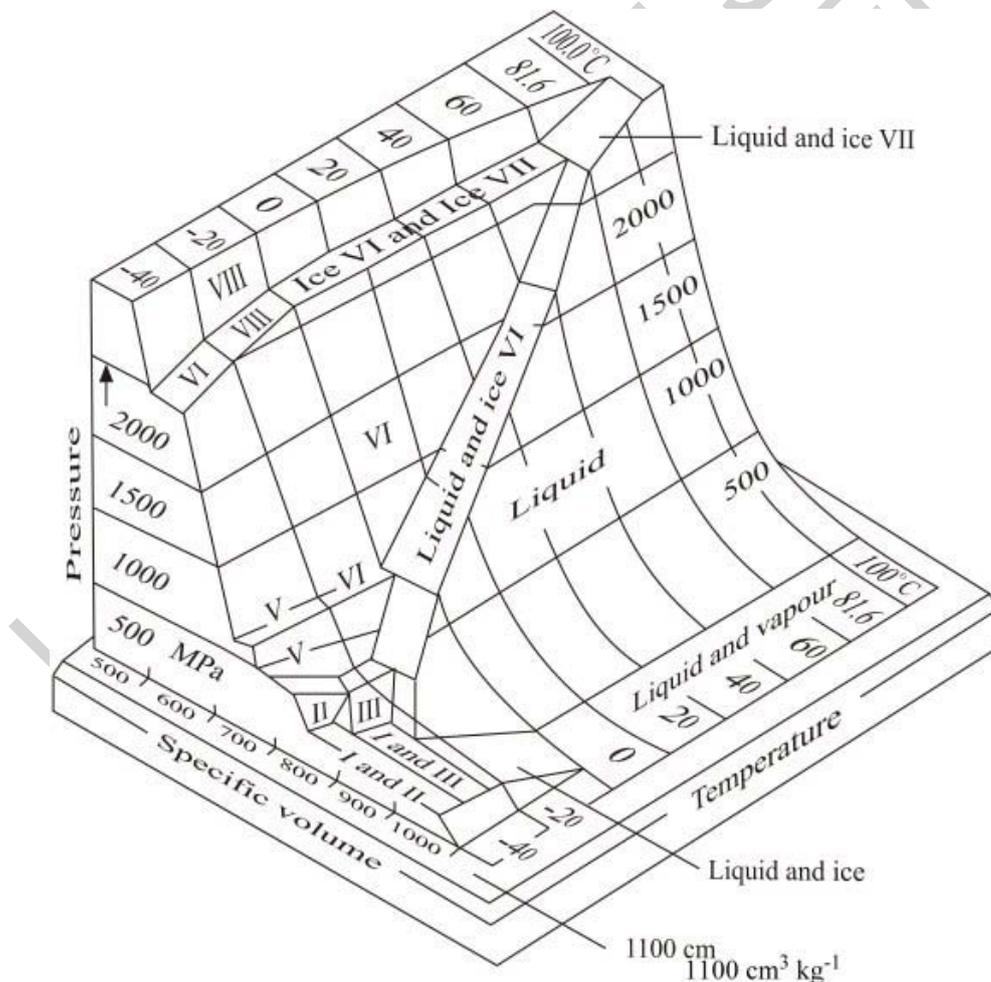
Figure 1. Surface “pressure - specific volume - temperature” for different ice variants and water
