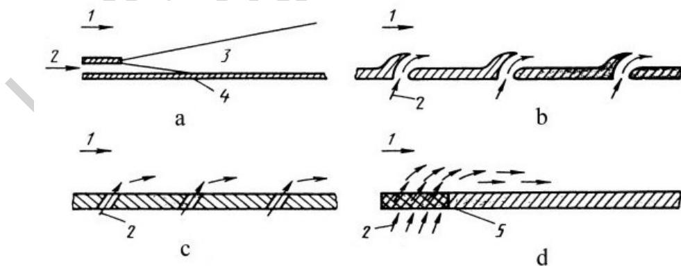
Figure 4: Schemes of coolant supply at block cooling of the surface: a – flat slit; b – system of slits; c – system of holes; d – porous insert; 1 - high-temperature gas flow; 2 – coolant; 3 – mixing region; 4 – protected surface; 5 – porous insert
