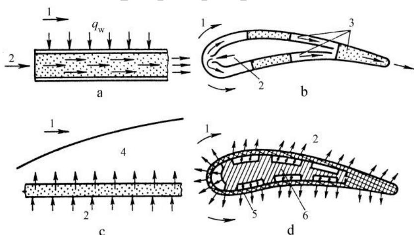
Figure 7: Schemes of porous cooling of protected surfaces: a – channel with a porous filler; b – cooled blade of the gas turbine with porous inserts; c – coolant injection into the boundary layer through the porous wall; d – porous cooling of the blade of the gas turbine with coolant blowing-out to its outer surface; 1 – high-temperature gas flow; 2 – coolant; 3 – porous inserts; 4 – boundary layer; 5 – porous wall; 6 – force rod
