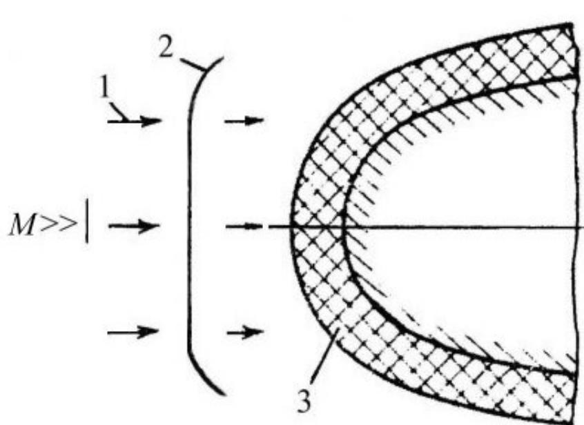
Figure 8: Schematic of the heat-protective coating of the frontal part of the flying vehicle: 1 – high-temperature gas flow; 2 – shock wave; 3 – heat-protective coating
