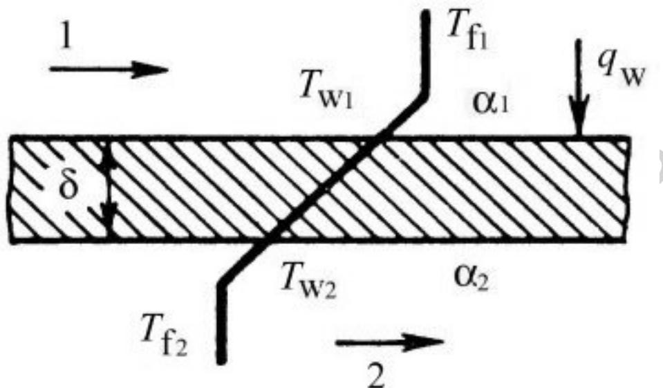
Figure 1: Convective cooling scheme: 1- high-temperature gas flow; 2 –coolant
