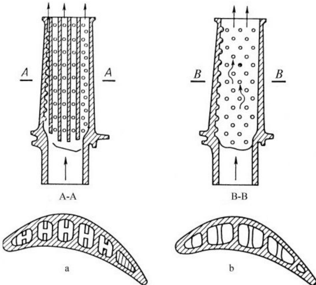
Figure 2: Methods of heat transfer enhancement in the channels of cooled gas turbine blades: a - fins; b – cylindrical intensifiers
