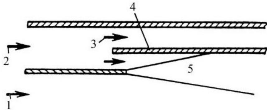
Figure 5: Scheme of combined cooling of the flame tube wall of the combustion chamber; 1 – high-temperature gas flow; 2 – coolant; 3 – convective cooling; 4 –flame tube wall of the combustion chamber
