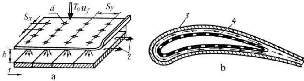
Figure 3: Jet cooling of the surface: a – jet cooling scheme; b – jet cooling of a gas turbine blade: 1 – high-temperature gas flow; 2 – coolant, 3 – outer casing; 4 –deflector
