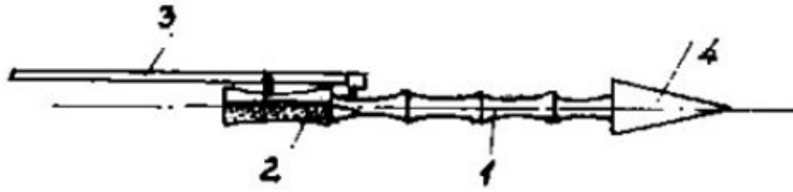
Figure 1. "Fiery arrows": 1- bamboo; 2- black smoky powder; 3- wooden pole for the stabilization; 4- stub
