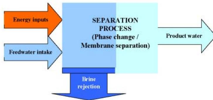
Figure 7. The basic principle of water desalination (Clayton, 2015).
