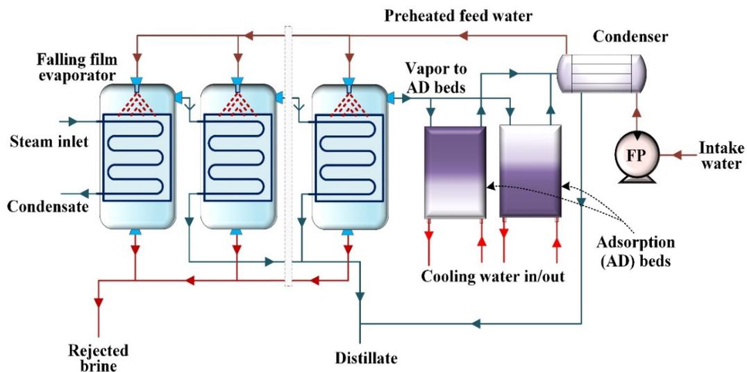
Figure 15. Multi-effect desalination hybrid with adsorption desalination system (Shahzad et al, 2014).
