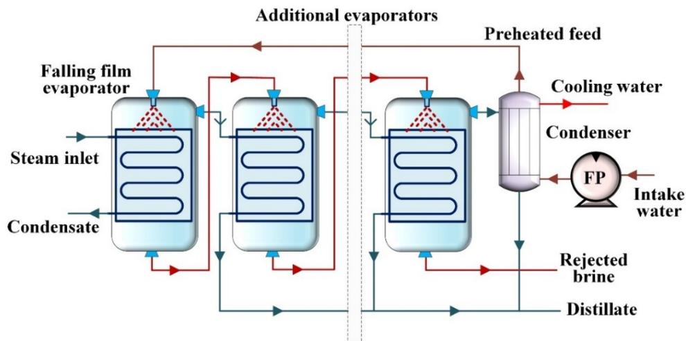
Figure 12. Forward feed MED system (Abid et al, 2020).
