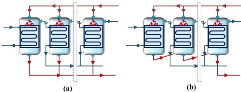
Figure 13. Multi-effect desalination evaporator arrangement for (a) parallel and (b) parallel cross feed arrangements (Elsayed et al, 2018).
