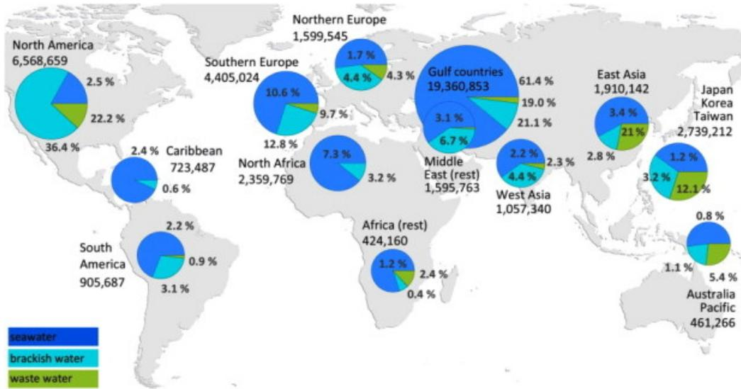
Figure 3. Global desalination capacities based on feed water quality (Ghaffour et al, 2013; Elimelech and Phillip, 2011).
