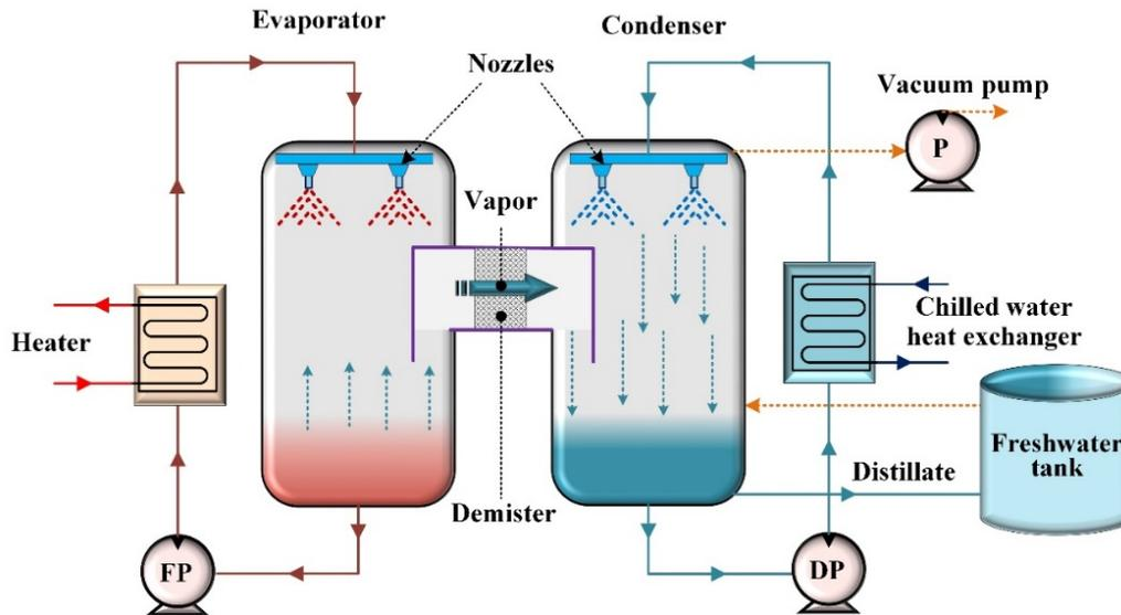
Figure 16. Direct-contact spray evaporation and condensation process (Qian et al, 2020).
