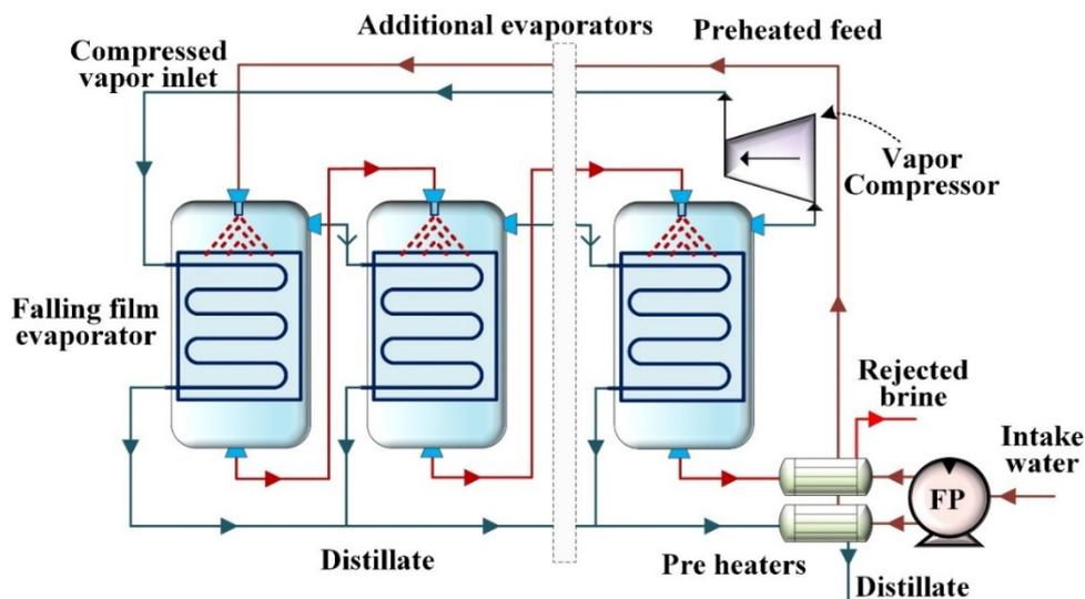
Figure 14. Schematic of MED-MVC system.
