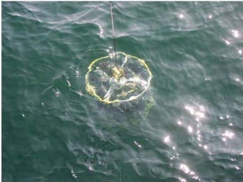
Figure 1. Conductivity-Temperature-Depth bathythermograph (CTD) lowered into the Baltic Sea for reading the local vertical profile of seawater properties. Photo taken on 25 March 2010 onboard of r/v “Prof. A. Penck”.
