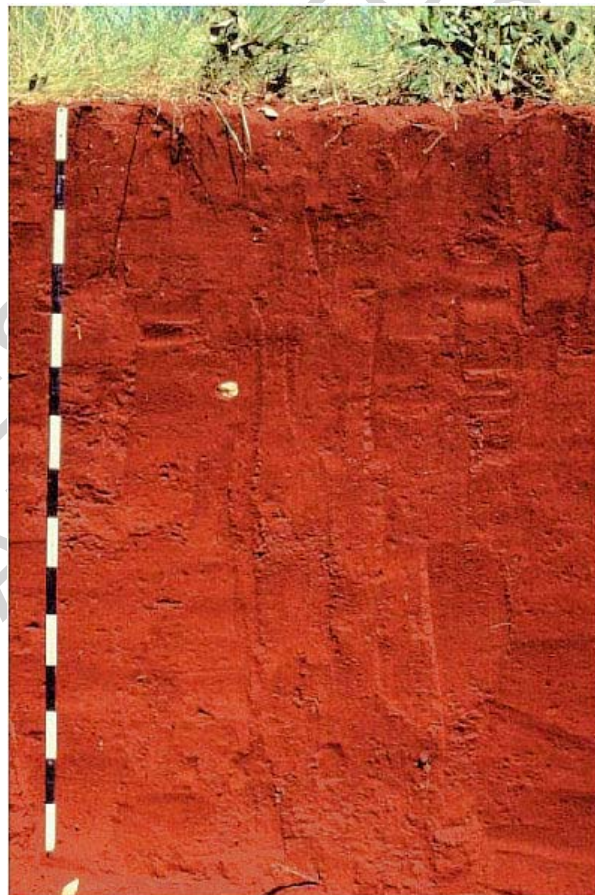
Figure 1. Ferralsol is the red-colored tropical soil with strong resistant microstructure (CD-ROM “Major Soils of the World”).
