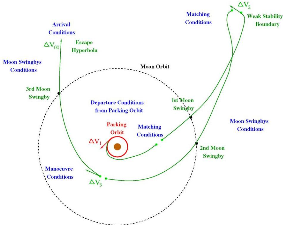
Figure 4. Example of a triple lunar swing-by Earth departure technique (obtained from Space Manifold Dynamics. Novel Spaceways for Science and Exploration)
