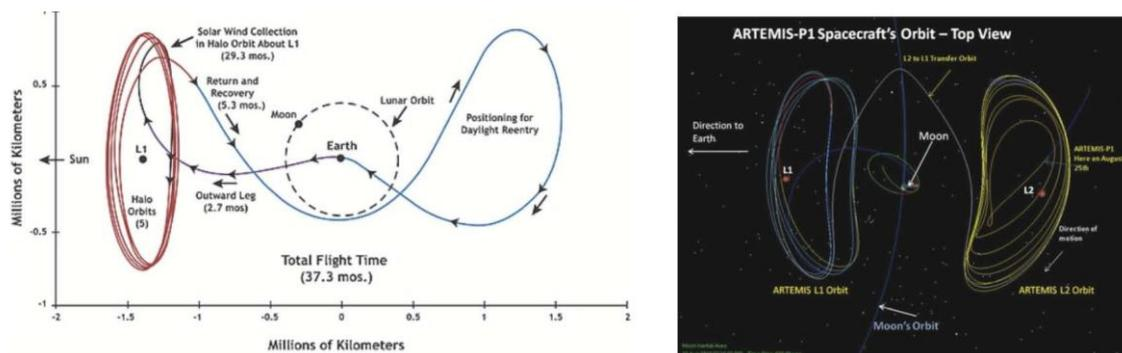
Figure 3. Left: Trajectory of the Genesis spacecraft. Right: Trajectory of the Artemis-P1 spacecraft following a heteroclinic connection in the Earth-Moon system. (From NASA's official web page).
