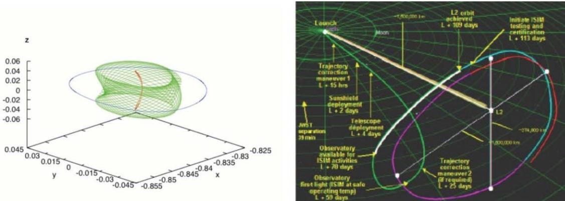
Figure 2. Left: A planar (blue) and a vertical (red) Lyapunov orbit, and a Lissajous orbit (green) for a fixed energy value around the equilibrium point  $L_1$ . Right: Nominal halo orbit (pink) and foreseen transfer orbit for the James Webb Space Telescope (from [http:// ngsc.gsfc.nasa.gov /](http://ngsc.gsfc.nasa.gov/)).
