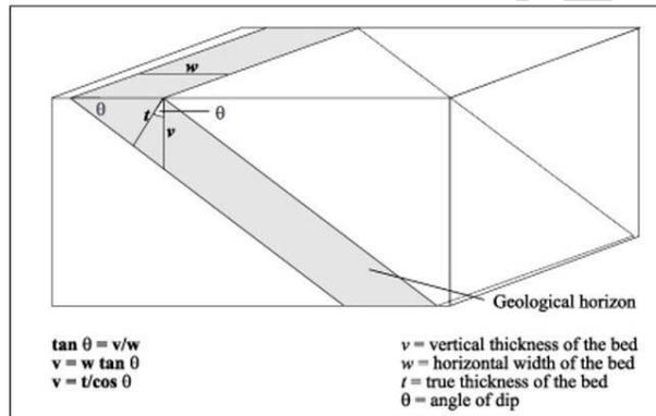
Figure 3: Determination of true thickness of a dipping bedding plane. Measuring the dip angle ( $\theta$ ) of the bedding plane and the width of the outcrop in the dip direction ( $w$ ) allows the true thickness of the unit to be determined by simple trigonometry.
