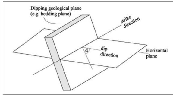
Figure 2: Basic geological terminology: dip and strike of planes. Although strike is commonly measured, the azimuth of dip is often favoured by some geologists - this is the bearing taken along the dip direction.
