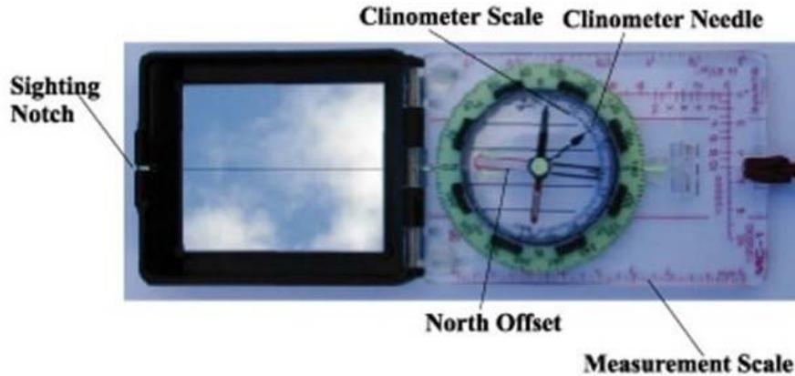
Figure 1: The basic compass-clinometer
