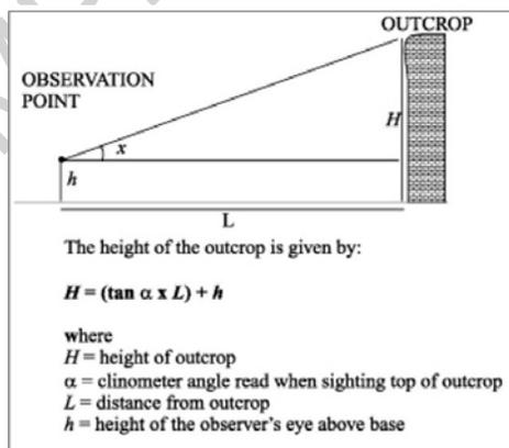
Figure 4: Calculating the height of an outcrop (cliff) using the compass-clinometer. Simple trigonometry and accurate sighting using the compass-clinometer allow heights to be rapidly determined.
