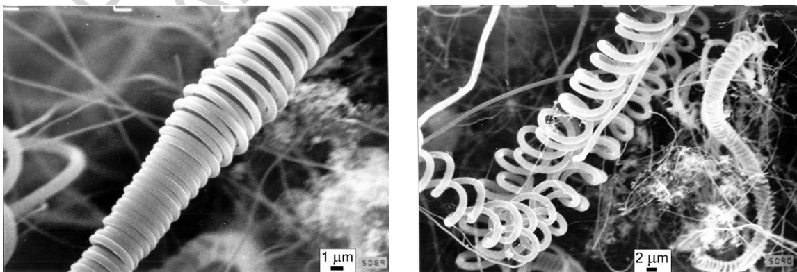
Figure 2. TEM images of the scroll-like gas-phase carbon fibers (Schur et al, 2007a) .
