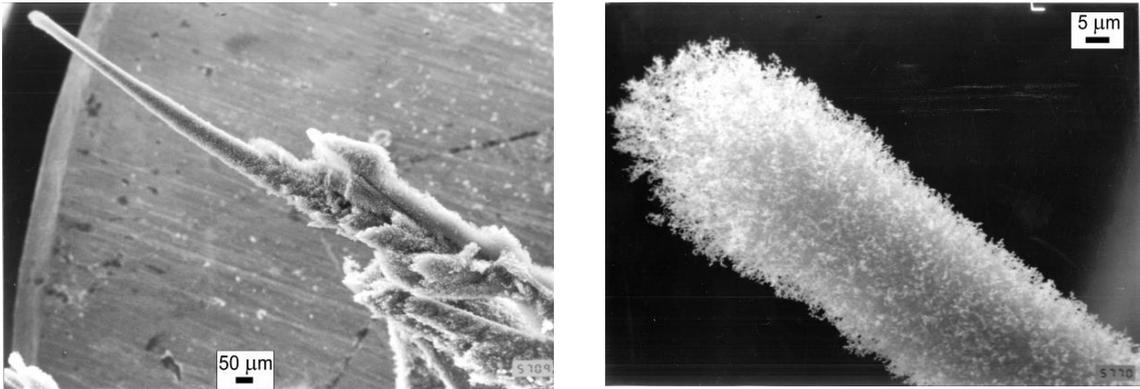
Figure 3. TEM images of the graphite whisker (Schur et al, 2007a)
