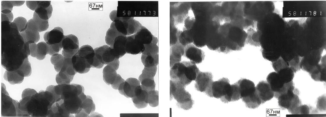
Figure 1. The photomicrographs of soot (transmission electron microscopy) (Schur et al, 2007a).
