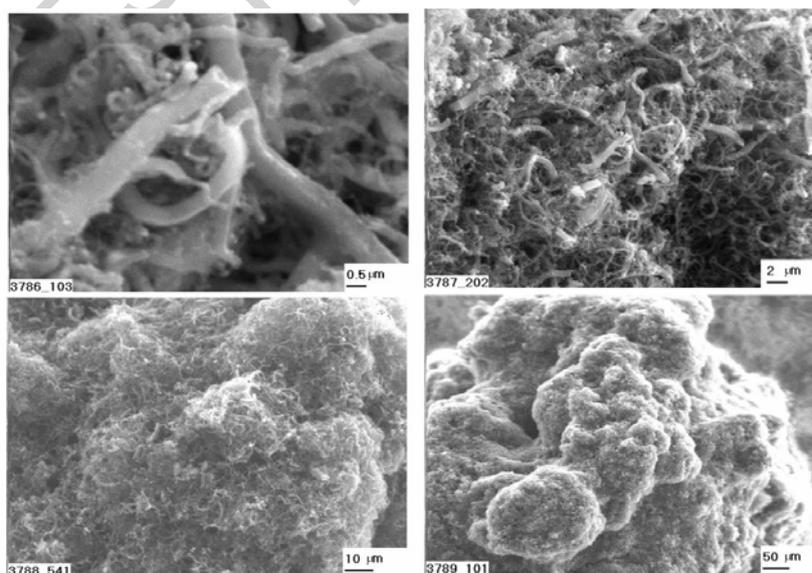
Figure 6. The fiber-based glassy carbon after the ultrasonic removal of amorphous carbon in toluene throughout 1 hour (Schur et al, 2007a).
