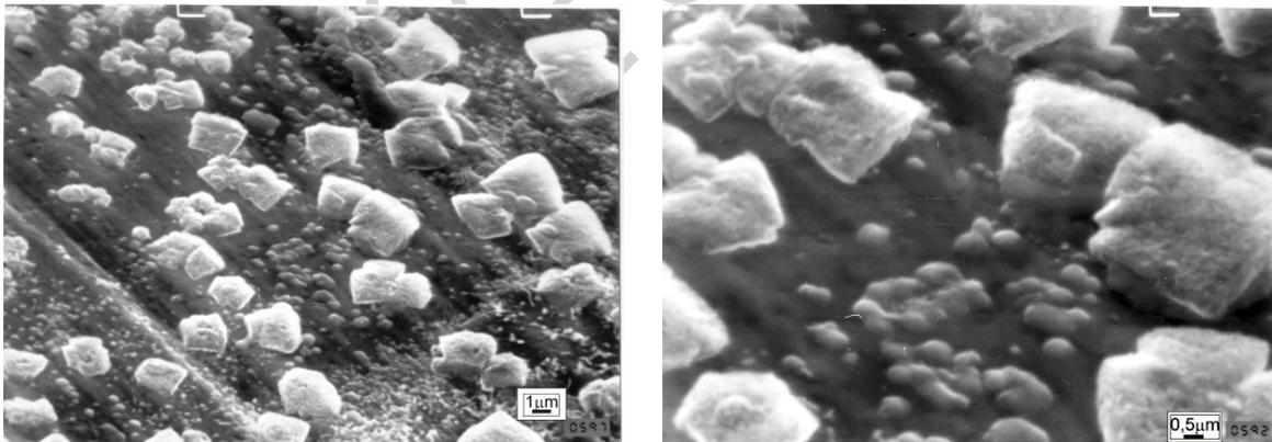
Figure 5. The nano- and microcrystals of diamond in the diamond-like carbon (Schur et al, 2007a)
