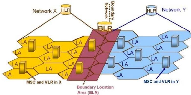
Figure 3: Boundary location register proposed for inter-system roaming
