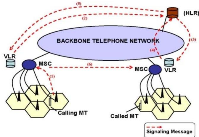
Figure 2: Call delivery in stand-alone cellular networks
