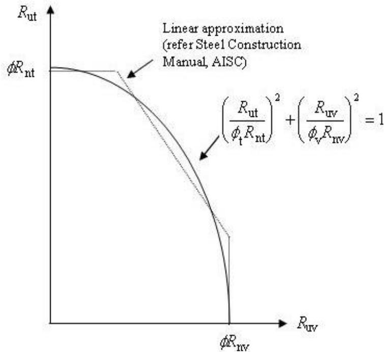
Figure 7. Interaction diagram between bolt shear and tension
