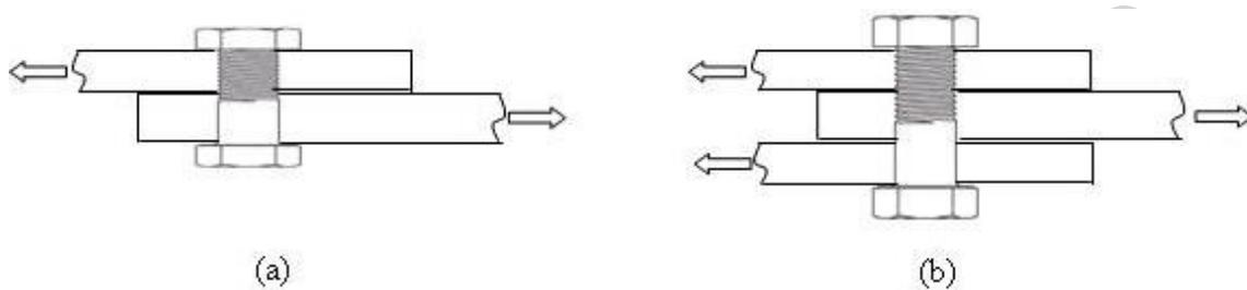
Figure 4. Lapped bolted joint (a) single shear and (b) double shear
