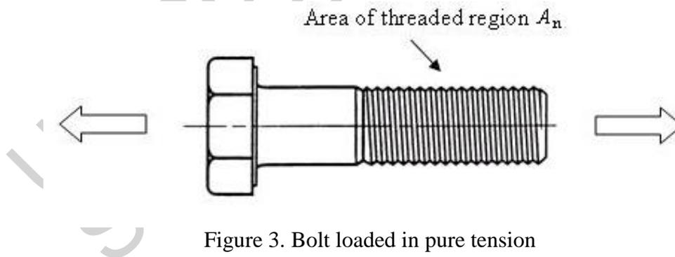
Figure 3. Bolt loaded in pure tension
