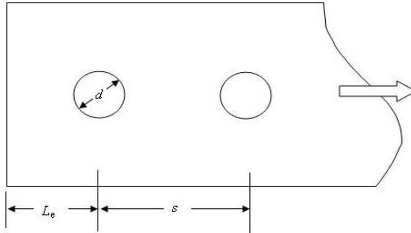
Figure 6. Bearing stress calculation for multiple bolt holes
