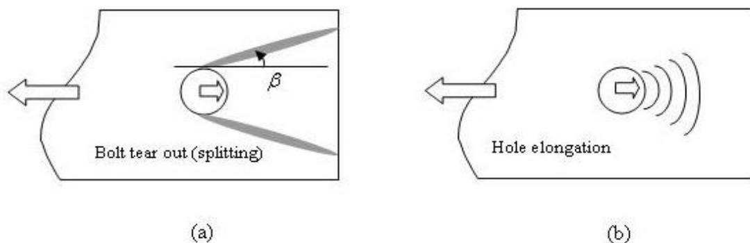
Figure 5. Bearing limit states at bolt hole
