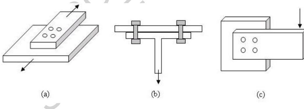
Figure 1. Types of bolted connections (a) Lapped tension splice (b) Hanger type connection (c) bracket type connection
