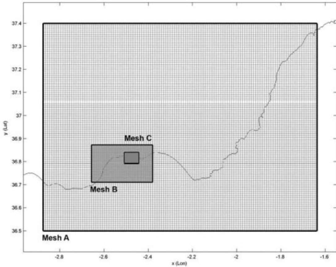
Figure 3. Location and size of the nested meshes used for the phase-averaged wave propagation model. Mesh A (500 m x 500m), Mesh B (100 m x100 m), Mesh C (50 m x 50 m)
