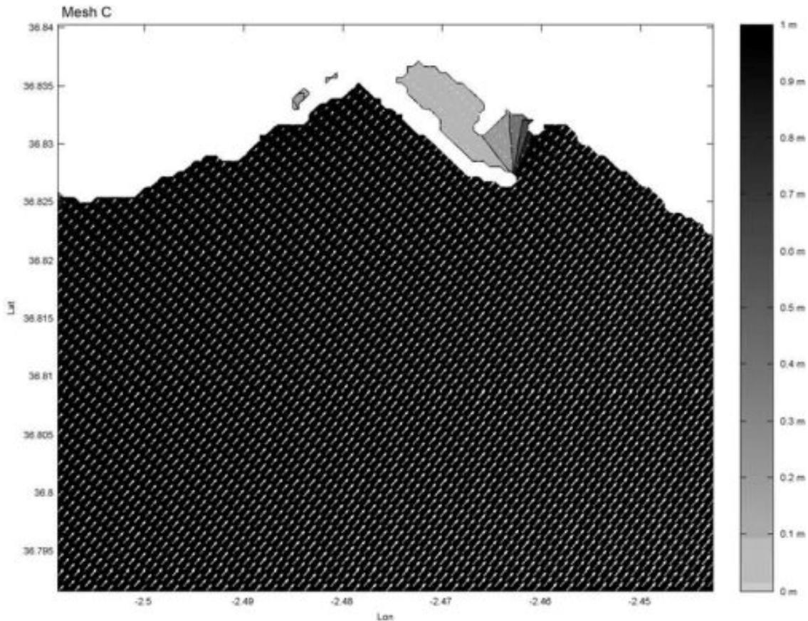
Figure 5. Wave height and direction for wave propagation calculated using the phase-averaged model SWAN at the Port of Almeria. Results are shown for mesh C and waves arriving from the southwest.
