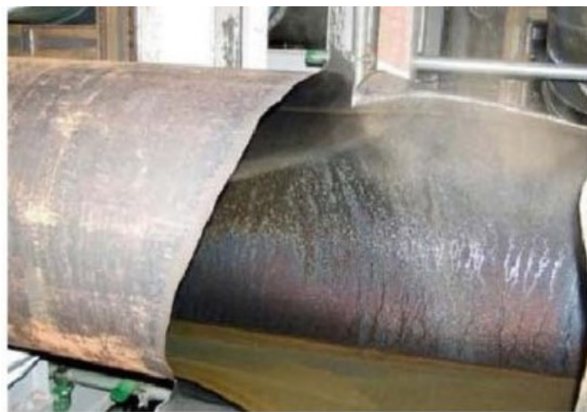
Figure 1. Pipe that ruptured at nuclear power plant after severe wall thinning at inner surface caused by flow-assisted corrosion.
