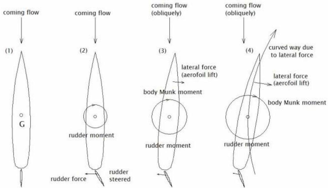
Figure 2. Schematic explanation of transition from straight running to turning
