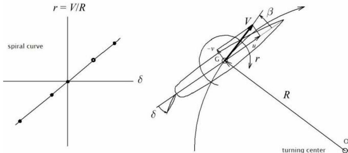
Figure 1. Steady turning state and spiral curve
