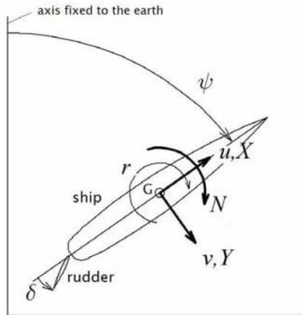
Figure 3. Coordinate system of maneuvering motion
