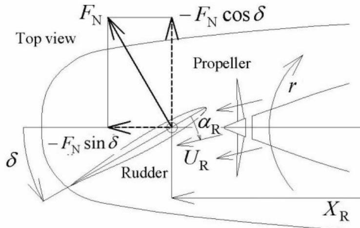
Figure 4. Rudder normal force
