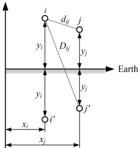
Figure 3 Application of the method of images.
