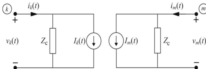
Figure 6. Equivalent circuit for time-domain simulations.
