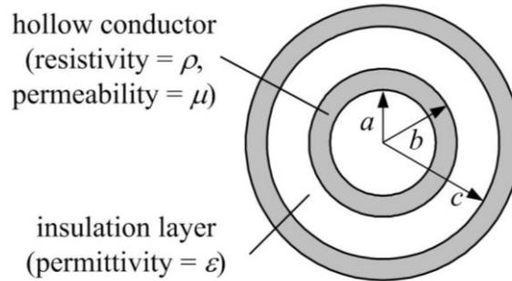
Figure 13. Cross section of a coaxial cable with a hollow conductor.
