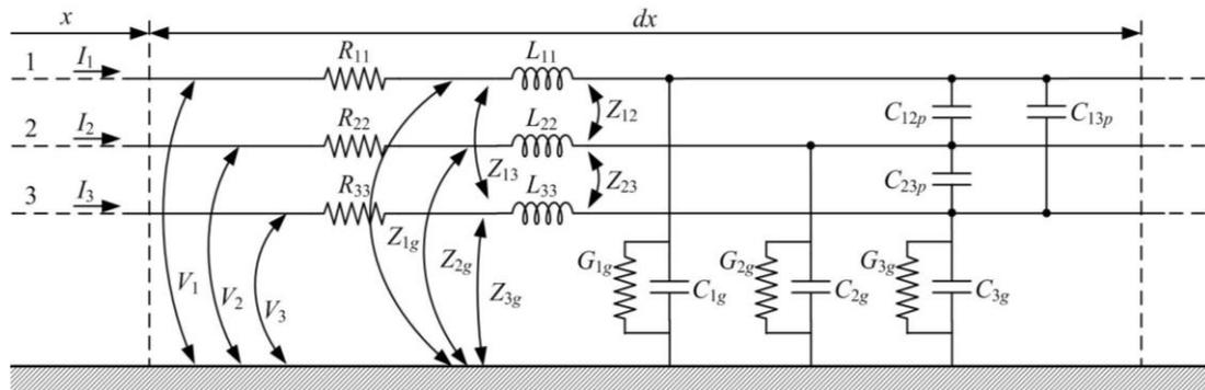
Figure 2. Differential section of a three-phase overhead line.
