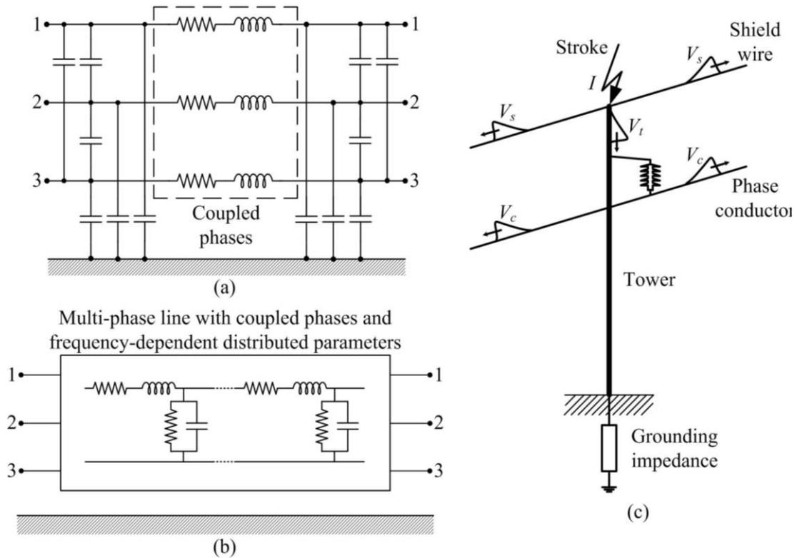
Figure 1. Line models for different ranges of frequency. (a) Steady state and low-frequency transients. (b) Switching (slow-front) transients. (c) Lightning (fast-front) transients.
