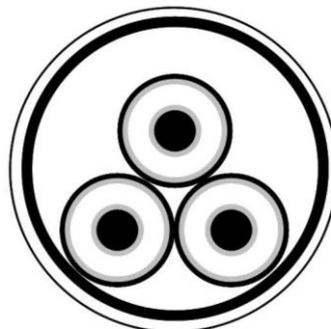
Figure 11. Pipe type cable.
