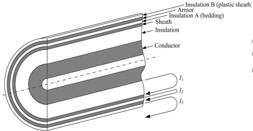
Figure 12. Cross section of a coaxial cable.
