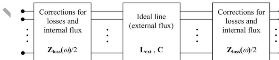
Figure 8. Section of a non-homogeneous line model.
