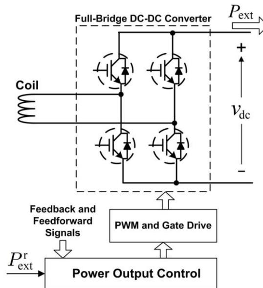
Figure 3. Schematic diagram of the conditioned energy resource for a SMES system
