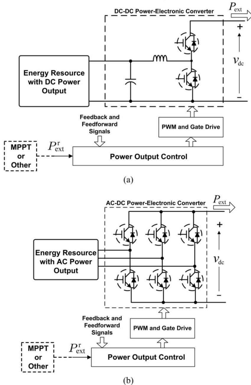
Figure 2. Generic schematic diagrams of (a) a conditioned dc energy resource, and (b) a conditioned ac energy resource
