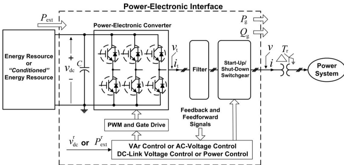
Figure 1. Generic schematic diagram of an electronically interfaced distributed energy resource (DER) system
