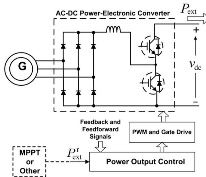
Figure 4. Schematic diagram of the conditioned energy resource for a small variable-speed wind energy system
