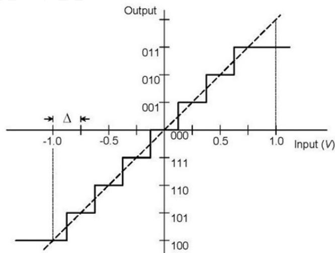
Figure 3. Input-output characteristic of an ideal 3-bit ADC with  $\Delta = 2/2^3 = 0.25$  V and
