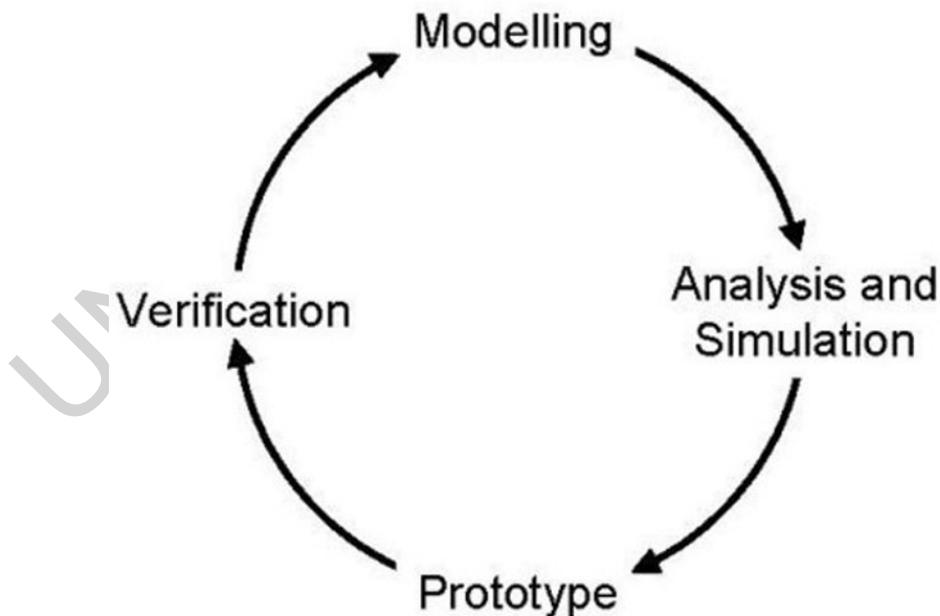
Figure 2. The engineering design cycle
