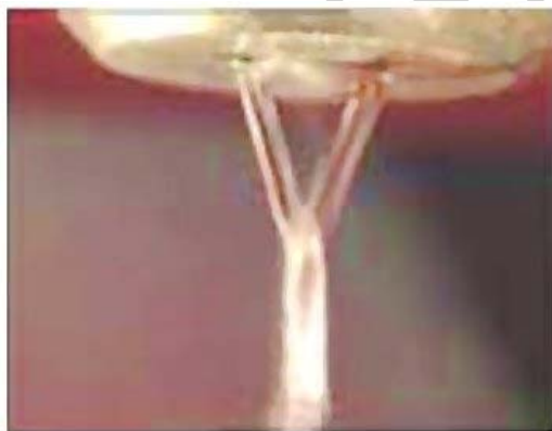
Figure 2: Stable y-type jets at the outlet of an impinging jet micromixer, (by courtesy of IMM).
