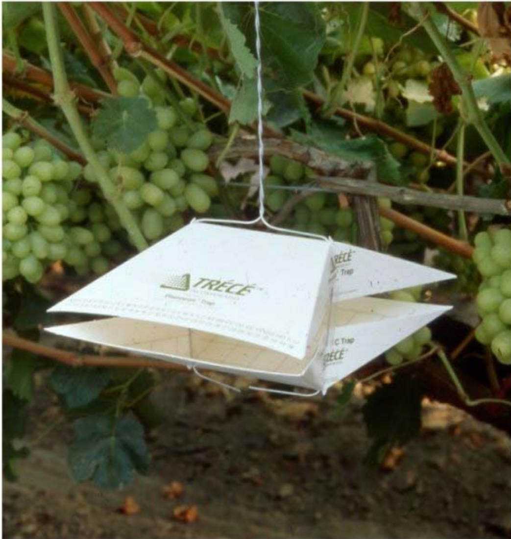
Figure 1. A typical pheromone trap used for insect monitoring purposes. The lower surface is coated with adhesive to trap insects attracted to the pheromone lure. (Image reproduced by kind permission of Trece Inc., USA)
