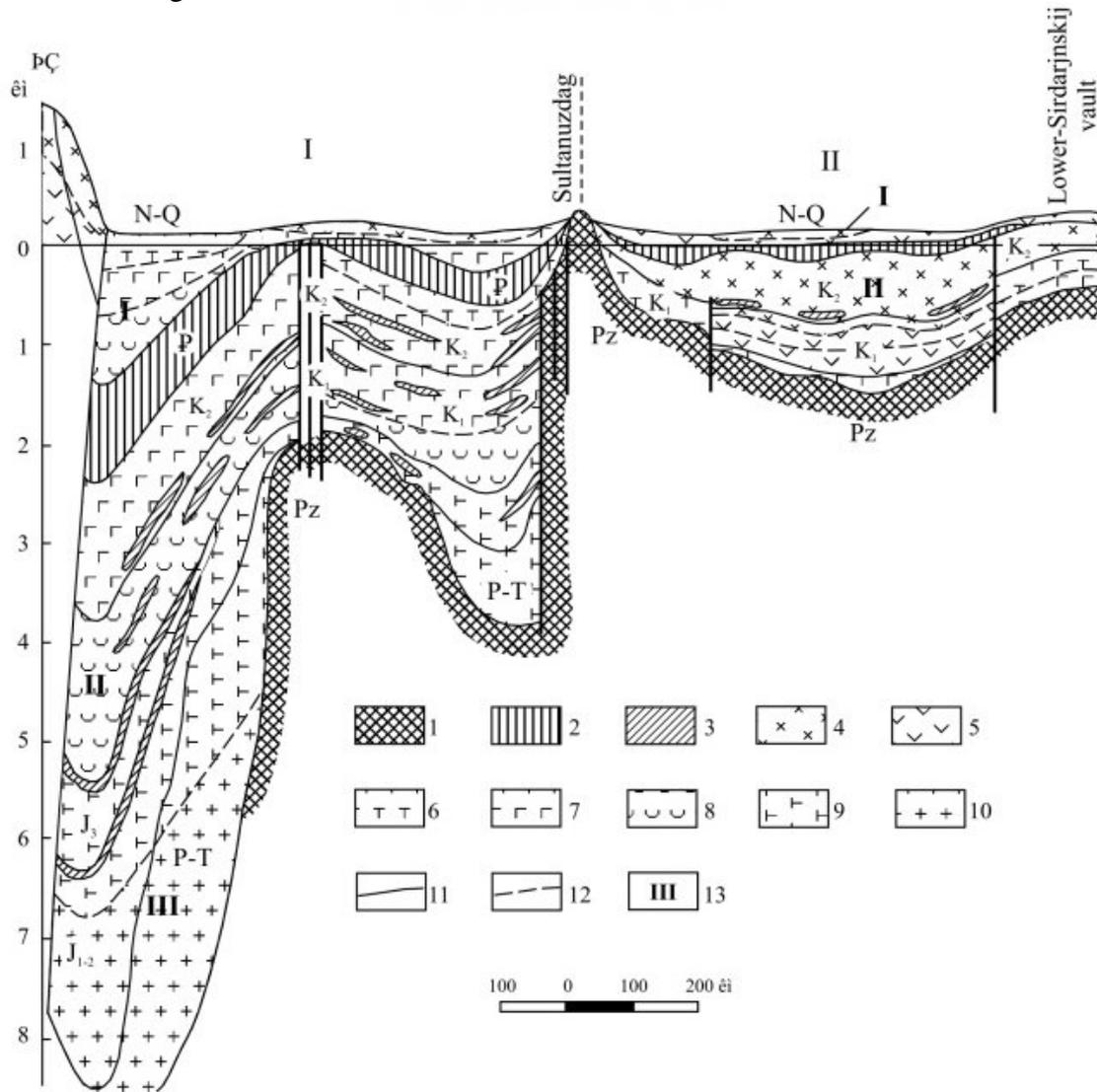
Figure 1. Hydrogeologic cross-section of artesian basins Turanskoj platform
