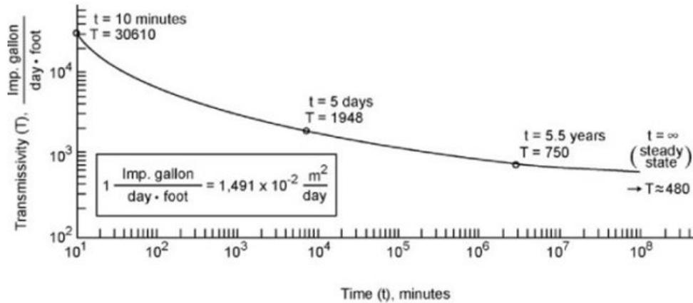
Figure 2. Transmissivities derived from pumping tests of increasing duration, and converging toward values obtained from basin-wide seasonal water-level fluctuations in a shale/sandstone rock framework (after Tóth, 1995, Figure 4)
