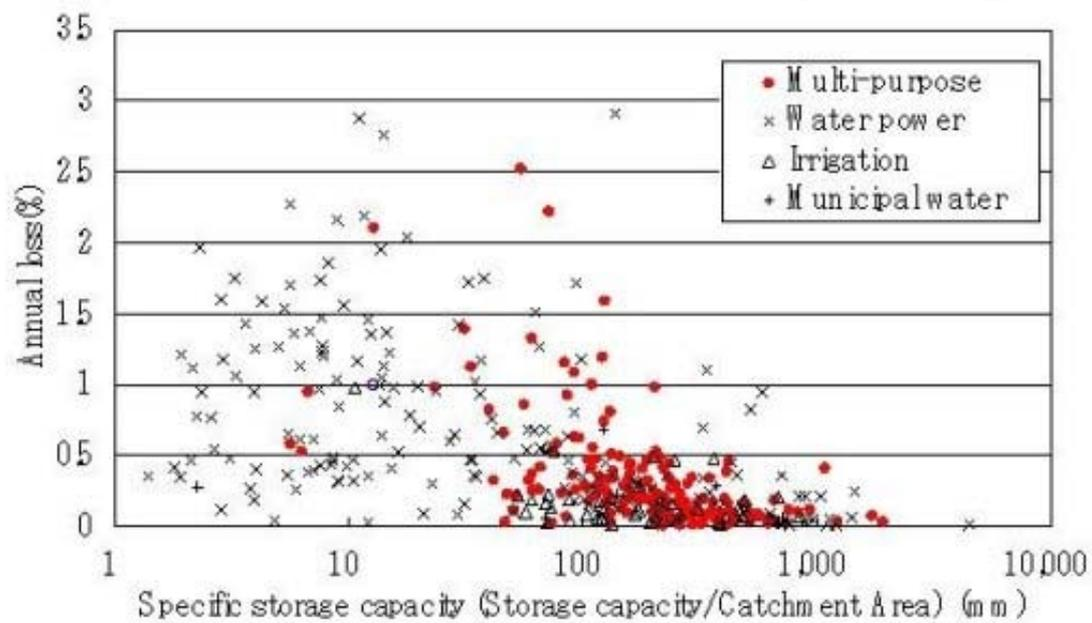
Figure 3. Specific storage capacity and annual loss in Japan
