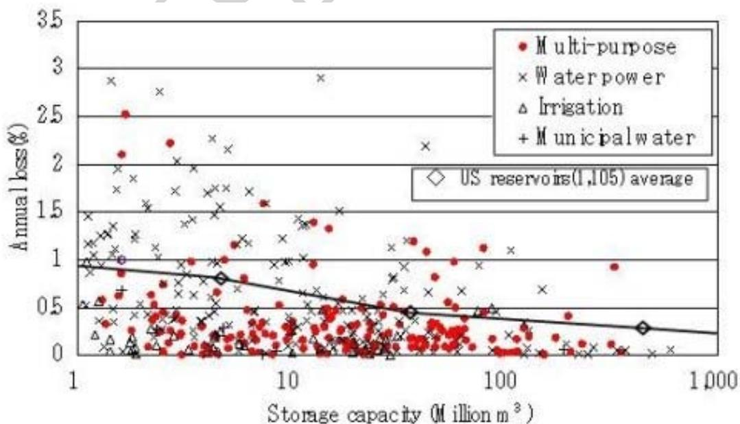
Figure 2. Reservoir storage capacity and annual loss in Japan
