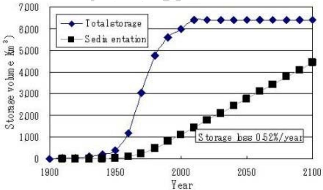
Figure 1. World storage volume and sedimentation loss
