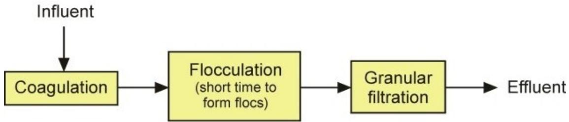
Figure 1. Process flow scheme of direct filtration
