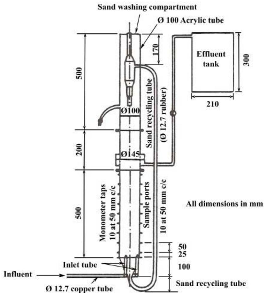
Figure 3. Sectional view of mobile bed filter
