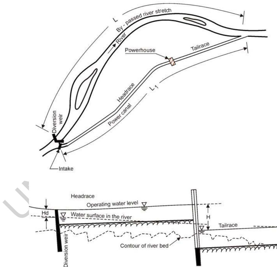
Figure 3. Profile of the diversion-type arrangement
