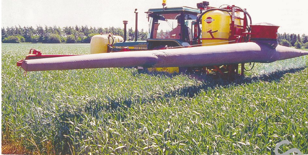
Figure 1. The PhytO3 Tech boom sprayer (Steffen, 2005)
