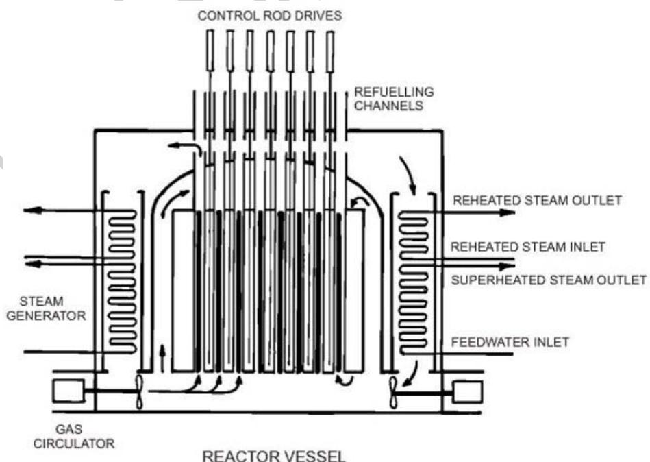
Figure 3: Diagrammatic cross-section of a typical AGR
