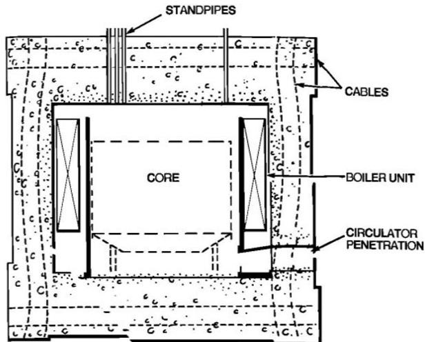
Figure 2: Magnox and AGR concrete pressure vessel with internal boilers
