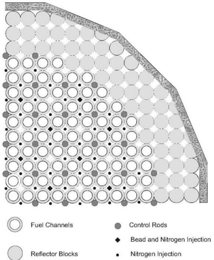
Figure 4: One quarter cross-section of reactor core
