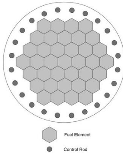
Figure 3: Dragon reactor core arrangement
