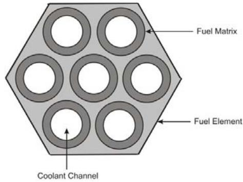
Figure 2: Dragon reactor fuel element cross section
